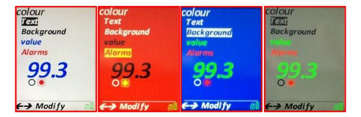
Pressing Up or Down cycles between the headings. Pressing Left or Right cycles through the available colours which are:
