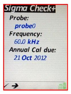
The selected Probe should be the same as what is actually connected to the instrument. If these differ then there is no guarantee that any values displayed will be accurate. If "No probe Info" is displayed, then a Probe needs to be selected from the *probe* menu, see 3.6.3 below.
