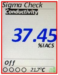
The Status Bar shows 4 Alarm LED representations, the temperature read by the probe, a MicroSD card icon and a Battery Meter or USB indicator.
